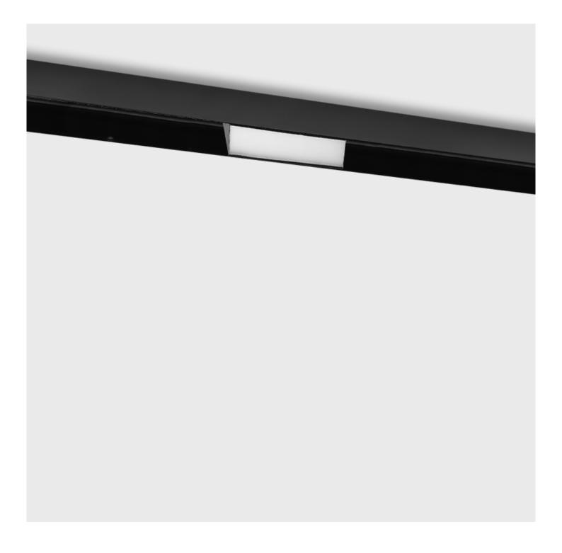
Modulo is a magnetic, LED track system in extruded aluminium with a range of versatile fittings available. The track is available in 2m lengths and can be interconnected via a connecting plate to form a recessed, surface mounted or pendant system. The power supply is remote. Opal is a recessed Modulo fitting in die-cast aluminium with opal diffuser, available in three sizes and wattages
